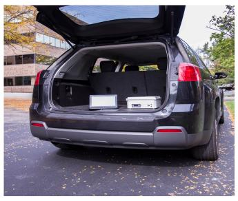
3DATX parSYNC® "integrated" PEMS (iPEMS) provide unique, hot-swap cartridges that deliver mass emissions – all in one compact 3.7kg unit (including batteries).
