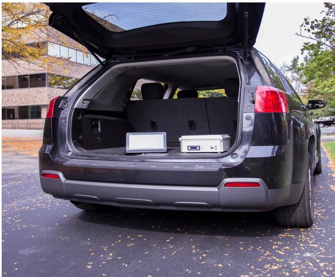
3DATX parSYNC<sup>®</sup> "integrated" PEMS (iPEMS) provide unique, hot-swap cartridges that deliver mass emissions - all in one compact 3.7kg unit (including batteries).
